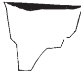
FIG. 3.—Transverse section of Loch Katrine. The black portion shows the true slopes; the outline shows the slopes exaggerated ten times.
